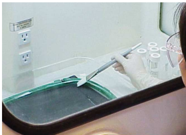
Fig. 2. Fabrication of a composite membrane for the fuel cell.
